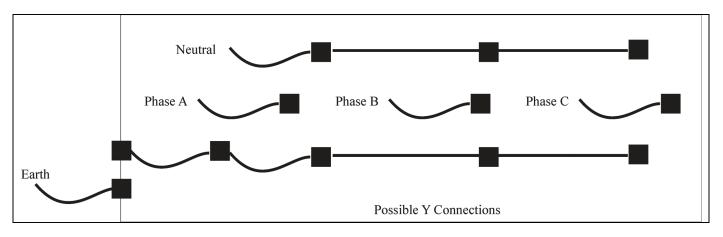
Each phase should be wired for a minimum of 15 A.
